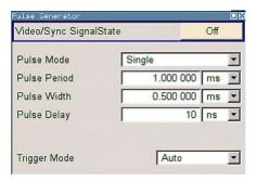
The dialog provides the settings for the pulse characteristics and trigger mode. Depending on the selected modulation source and pulse mode the provided parameters vary.
