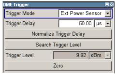
The "DME Trigger" dialog contains the parameters for configuring the trigger mode. If a connected R&S NRP-Z81 power sensor triggers the setup, the R&S SMA provides additional parameters for synchronizing with the sensor.
