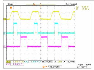
Channel 1 = Indicates the external trigger signal. The positive slope is active.
