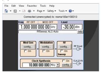
6. Use the mouse cursor and keyboard to access the functionality of the instrument as you would directly perform the settings on the instruments front panel.
