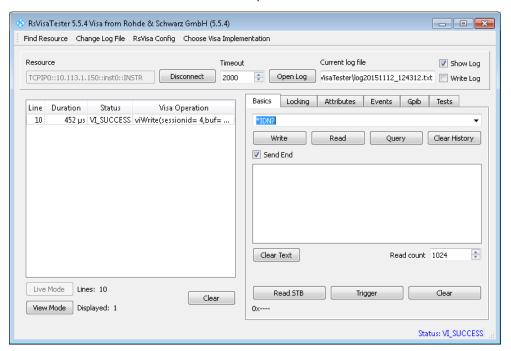
**Tip:** If the "Show Log" checkbox is checked R&S VISA displays each VISA function call in the log-view on the left. If you check the "Write Log" checkbox the log-view entry is written to the log file as well. You can operate the log-view in two modes: the "Live Mode" shows only the most recent messages whereas the "View Mode" allows you to scroll the history.
