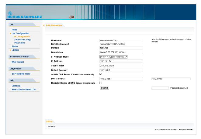
The "IP Address Mode" selects a configuration mode for the IP address of the R&S SMA. With static configuration, the entered IP address, subnet mask, and default gateway are used. With dynamic configuration, DHCP or dynamic link local addressing (automatic IP) are used to obtain the instrument IP address.
