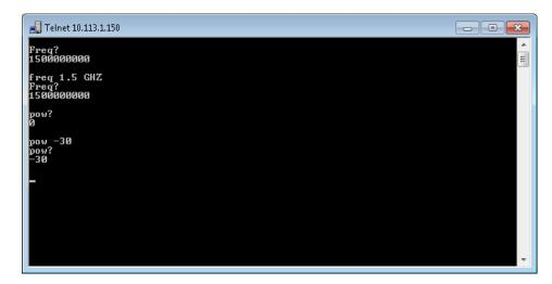
After the first remote-control command has been sent, the instrument is in the "REMOTE" state, i.e. instrument control from the front panel or via mouse and keyboard is disabled and "REMOTE" is displayed in the status line.
