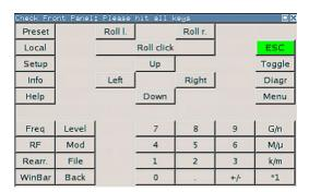
Reflecting the front panel, the "Check Front Panel" dialog contains all functions to test the operating elements of the instrument.
