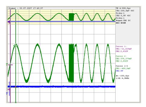
Figure 5-2: Transition for a 1 kHz step at 1 GHz without phase continuous mode active. For the graphical display the signal is down converted into the kHz range.
