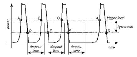
As the mechanism associated with the dropout time parameter is reactivated whenever the trigger threshold is crossed, unambiguous triggering can also be obtained for many complex signals. By contrast, all triggering is suppressed during the hold-off time. I.e. in the example, that although stable triggering conditions can be obtained with a suitable hold-off time (regular triggering at the same point), it is not possible to set exclusive triggering at A.
