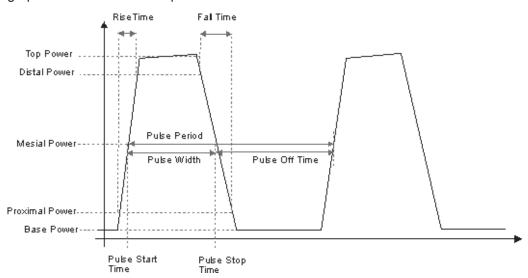
The sensor calculates the pulse parameters from each measurement and delivers the results to the R&S SMA.
