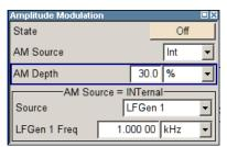
e) Finally, select "State" and press the rotary knob to switch on the AM modulation.
