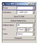
With the **reference** and **hold** traces, you can compare traces. Assign a reference curve to one trace and your measured values to a second one, and switch on the display. This feature provides to compare results directly in the graph, or to show deviations in a graph by using the "Mathematics" function.
