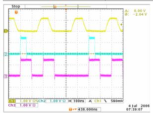
Channel 1 = Indicates the external trigger signal. The negative slope is active. A second trigger signal during double pulse generation is without effect.
