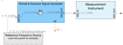
Figure 5-6: Synchronizing a subsequent instrument an externally applied reference frequency of 5, 10, or 13 MHz
