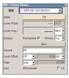
The dialog shows the settings and measurement values of the sensor selected in the field next to the connector symbol. For indicating the parameters of another sensor, switch to the respective sensor in the selection list.
