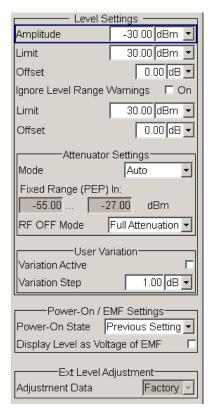
The offset-free level, level offset and level limit are set in the top section of the dialog. The attenuator mode is set in the "Attenuator Settings" section.
