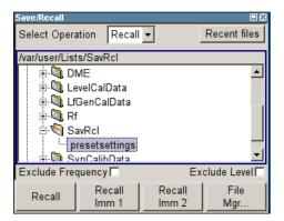
The available drives and directories and the files of the selected directory are displayed. The currently selected path is displayed above the window. Only the relevant files without file extensions are displayed. If the area is opened several times, the path last selected is displayed. When a file is saved or created, its name is user-selectable; the extension is assigned automatically and cannot be entered. The file is saved to the selected path.
