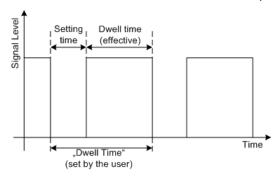
The "Dwell Time" set by the user is used as the step time of the sweep. The effective net dwell time is shorter, reduced by the setting time. This setting time may be greater than the time specified in the data sheet.
