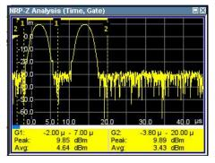
The start and stop time of the gates are indicated as gate markers, a bar between the start and stop marker shows the gate length. The indication state of the gate borders and measurement values is only available for certain diagram views which are switched with the "REARR" key. The "REARR list NRP-Z Analysis" dialog provides a selection of views, between which is toggled (see "REARR list - Power Analysis" on page 199).
