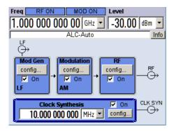
Figure 3-1: Block diagram of a fully equipped R&S SMA
