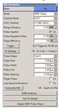
The "DME Modulation" dialog contains the channel, pulse pair and trigger parameters, and the parameters for setting the modulation. To measure the "Reply response", use an R&S NRP-Z81 Wideband Power Sensor.
