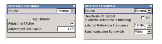
In the "Reference Oscillator Settings" dialog, you can select the signal source and frequency to be used as the reference frequency, and determine a user-defined adjustment value.
