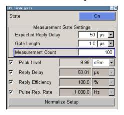
The "DME Analysis" dialog provides the settings to configure the parameters of the reply signal of the ground station transponder. You can use this feature when an R&S NRP-Z81 power sensor is connected to the R&S SMA sensor connector.
