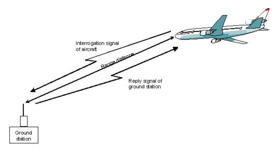
The DME channels are paired with the VOR frequencies, in the range between 1025 MHz to 1150 MHz for the interrogator, and 962 MHz and 1213 MHz for the transponder. The spacing for all channels is 1 MHz. X and Y channels differ in the spacing between the two pulses of the pulse pair and in the delay for the reply pulse.
