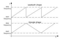
"Sawtooth" The sweep runs from the start to the stop frequency. Each subse-
