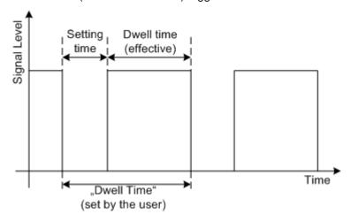
The "Dwell Time" set by the user is used as the step time of the list mode. The effective net dwell time is shorter, reduced by the setting time. This setting time may be greater than the time specified in the data sheet.
