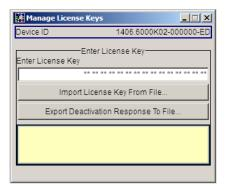
An option is ready to operate after it is enabled by means of a license key code supplied with the option. The license key is delivered as a file or on paper. Unregistered licenses must be registered for a particular instrument prior to the corresponding option can be enabled for operation.
