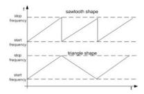
"Sawtooth" One sweep runs from start to stop frequency. Each subsequent
