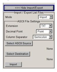
Externally edited Excel tables with frequency/level pairs can be imported as text or CSV-files and used for list mode.
