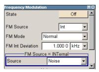
Gauss distribution and full bandwidth (10 MHz) are the default settings for the noise signal. These settings are not changed.
