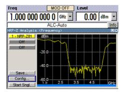
The R&S SMA supports various graph views, according to the methods of measurement and also additional functions such as the use of markers.
