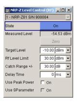
The dialog contains all parameters for configuring the settings for level control test setup.
