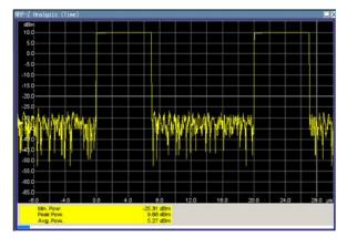
"Minimal / Peak / Average Power" display the minimum, the maximum and the average power of the pulse signal in dBm.
