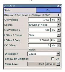
The dialog provides access to the configuration of the internal modulation generators, and you can activate the output of the LF signal
