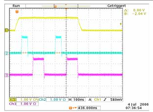
Channel 1 = Indicates the external gate signal. The signal is active when it is high (positive).
