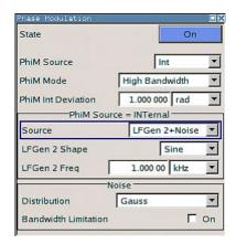
In the upper section of the dialog, the modulation source is selected and the modulation switched on. The modulation source can be selected independently for the different modulation types and the LF output.
