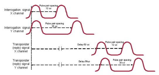
Figure 5-12: Timing of the pulse pairs (slant range distance = 0 nm)
