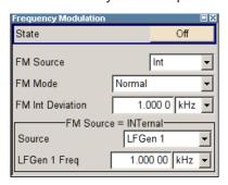
The internal source is the LF generator 1 by default. This setting is not changed.
