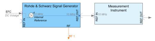
Figure 5-4: Synchronizing a subsequent instrument using the internal 10 MHz reference signal of the R&S SMA
