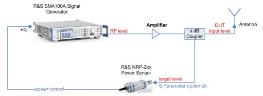
Figure 5-7: Example of a test setup with NRP-Z Level Control
