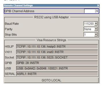
The "Remote Channel Settings" dialog contains the GPIB address and displays the VISA resource strings provided for remote control via the various interfaces.
