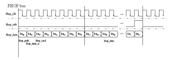
Figure 5-11: Input control signals for List Modes Fast Hop and Fast Hop Direct on the serial FHOP bus
