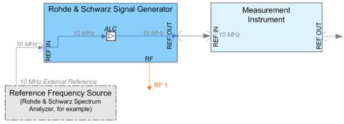
Figure 5-5: Synchronizing instruments by means of an externally applied reference signal having 10 MHz
