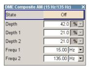
The "DME Composite AM" dialog provides the settings for a two-tone signal that can be superimposed on the DME pulses with amplitude modulation. This feature enables you to simulate the variation of the DME pulse amplitude for DME receiver testing.
