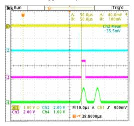
Figure 5-14: DME reply CH X (Trigger = External)
