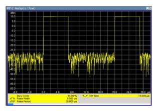
"Duty Cycle" Indicates the ratio between the pulse duration (τ) and the pulse period (T) of the measured pulse signal in per cent:
