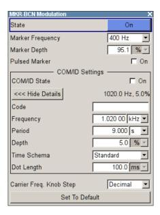
The "MKR-BCN Modulation" dialog contains the parameters for configuration of the marker, and the COM/ID settings for the modulation.
