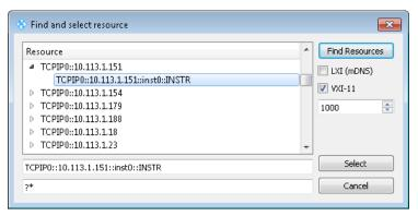
The "Find and select resource" dialog closes and R&S VISA indicates the instruments IP address in the "Resource" field of the main application window.
