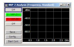
The measurement data of the sensors is displayed in traces in a measurement diagram. Four traces are available. The traces are automatically or manually assigned to the sensors. In addition to the data traces, a reference trace can be stored and recalled and/or the trace indication can be frozen temporarily (hold trace), thus enabling comparison of traces. Readout and comparison of particular values of the traces is possible by means of four markers.
