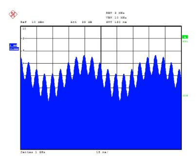
Figure 5-15: Measurement of RF envelope with DME interrogations at 6000 pp/s
