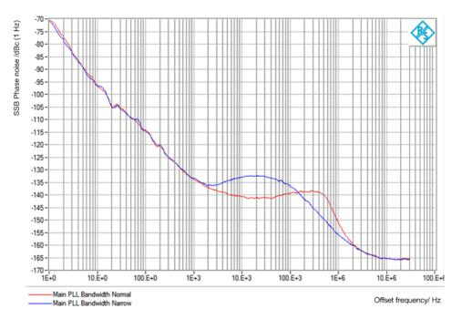
Figure 5-1: SSB Phase Noise, comparison of the main synthesizer PLL bandwidth "Narrow" and "Normal"
