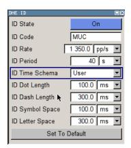
The "DME ID" dialog contains the parameters for configuring the identification sequence for the reply signal. Each airport identifies itself with a three letter code, for example 'MUC' for the Munich airport. This information is transmitted in Morse code. The transmission of the identification sequence can be suppressed.
