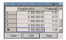
"Frequency / Hz" Enters the frequency to which the level correction value applies.
