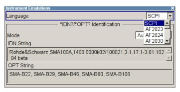
The "Instrument Emulations" dialog enables you to emulate a remote control command set of several other signal generators.
