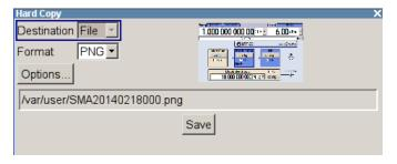
The dialog contains the parameters for configuring the output format and location of a hardcopy.
