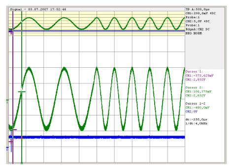
Figure 5-3: Transition for a 1 kHz step at 1 GHz with phase continuous mode active. For the graphical display the signal is down converted into the kHz range.
