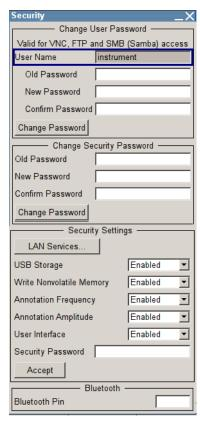
The "Security" dialog comprises the parameters for configuring the passwords, as well as the security settings of the mass storage and the LAN services.
