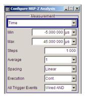
The measurement section provides the parameters for configuring the measurement either in frequency, power or time domain.
