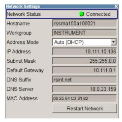
In the "Network Settings" dialog, you can configure the settings of the general network environment and specific identification parameters of the instrument in the network.
