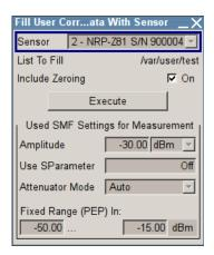
This dialog describes all parameters for filling a table automatically with sensor readings.
